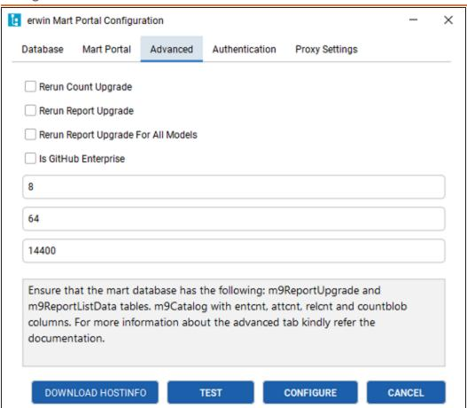
In case of failures in upgrade, before you rerun the upgrade, on the Advanced tab, configure the following settings:
