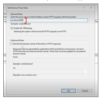
11. Under Inbound Rules, add the server name or the IP address and port number of the server where you have installed and configured erwin Mart Portal.
